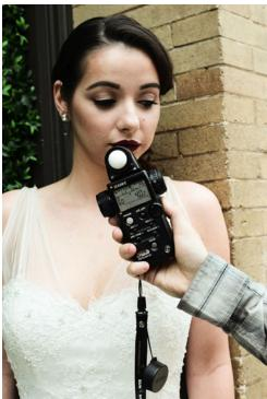
Figure 4 - Using a flash meter is a great way to quickly and accurately read the percentage of light contributed by the flash. 20% to 30% is the perfect range for creating a natural-looking fill-flash balance between flash and ambient.
